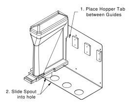
3. To operate the Dispenser, place a container under the spout. Push the Slider to dispense product. Pull the Slider back to reset for the next dispense.
