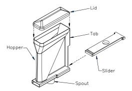
Place an assembled Hopper onto the Mounting Bracket. The Tabs on the back of the Hopper fit underneath the edges of the Mounting Guides.
